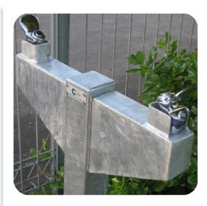
Installation of all models needs to be made near a 15mm mains pressure potable water supply (with an in-line pressure limiting valve – 105PSI Max). It also needs a well drained concrete surface area for excess water run-off
