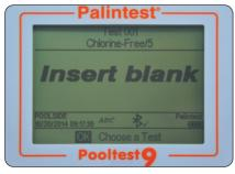
Insert the Blank cuvette and press OK.
