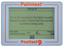
Ensure the blank cuvette is being used, not the sample plus reagent cuvette. Sample colour can be reduced by dilution with clean water; the dilution selected should take account of the expected concentration of parameter under test. Blank results are stored in the temporary memory of the Pooltest 9 and will be used for all subsequent tests until:
