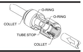
Pull on the fitted Tubing to ensure it is secure. Tube should not come free from the Fitting. Water test the connection assembly prior to leaving the site to ensure there are no leaks.
