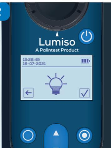
Use the up and down keys
