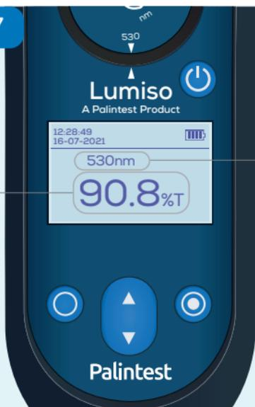
The measurement of %T (Percentage Transmission) is shown on screen.
