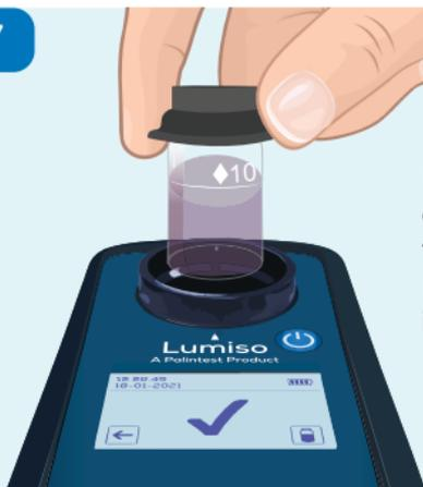
Prepare a 10mL sample by adding reagents according to the test instructions. Place this sample tube in the cell holder.
