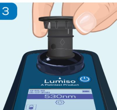
To set the blank (zero) value for the selected wavelength. Insert the "Blank" from the set of standards.
