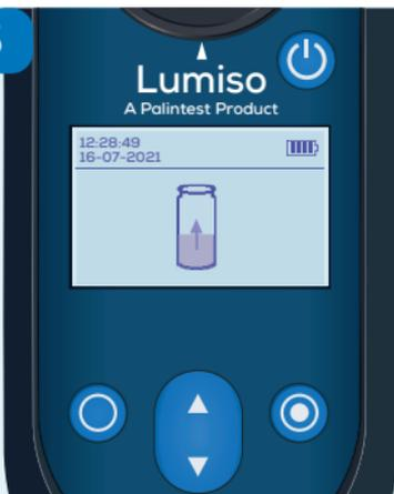
The screen will show that the blank is being measured.
