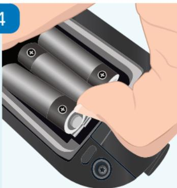
The batteries are held firmly in place by the clips to enhance Lumiso's resilience to physical shock.
