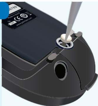
To change the batteries, first disconnect the USB lead.
