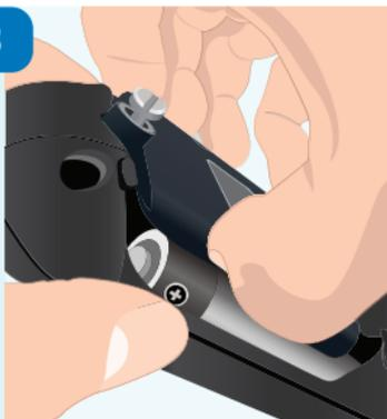
The cover will lift and, if necessary, the captive screw can be further loosened so the cover can be removed completely.
