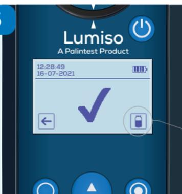
The instrument will measure the blank and show when this has been successful.
