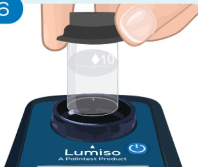
Ensure that your Lumiso Instrument is clean and dry. Place tubes in the instrument with white diamond aligned to the mark on the instrument.
