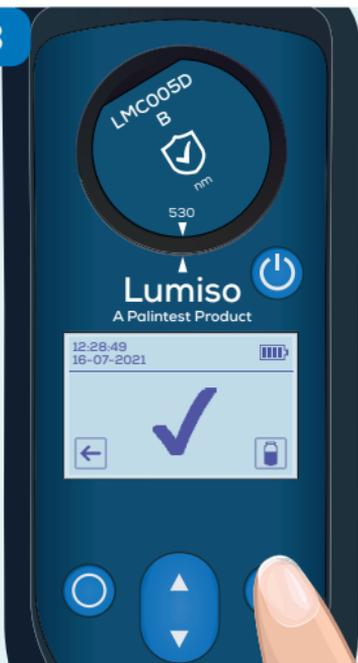
Continue, by inserting all the remaining standards, pressing read, and comparing the result with certificate.
