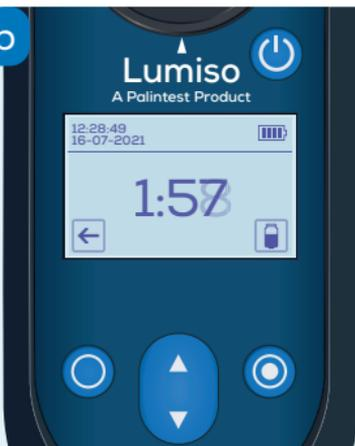
For tests with a "wait time" (see test instructions), a preset timer will count down and then automatically commence reading.
