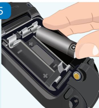
Insert new batteries in the same way, pushing towards the negative contact, but this time, down at the positive end.
