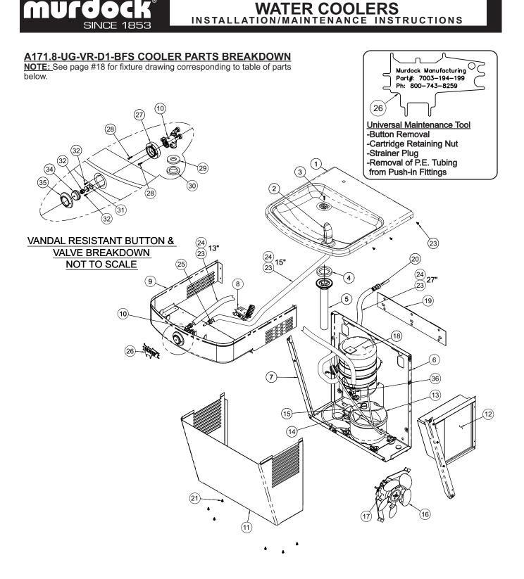
Standard A171.8-UG-VR-BFxS series refrigerated ADA cooler shown. All 1/4" O.D. Plastic tubing (23) must be insulated with (24) foam insulation.
