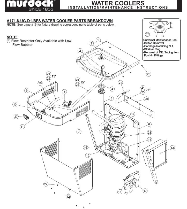
Standard A171.8-UG-BFxS series refrigerated ADA Water Cooler shown. All 1/4" O.D. Plastic Tubing (24) must be insulated with (25) foam insulation.
